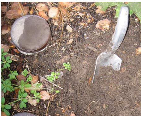
Figure 6. A metal spade is a good choice for soil sampling in softer soils. Metal spades have few crevices which makes them easier to sterilize between samples. In this planting basin, the plant had recently died but the soil was tested.
