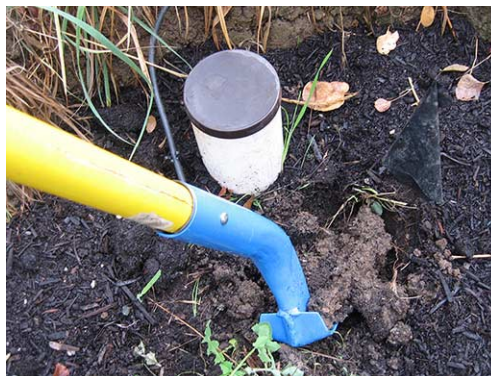
Figure 7. A trenching shovel maybe used for sampling harder soils. Its narrow profile facilitates sampling soil associated with restoration plants without harming too many roots, and it can be applied forcefully.
